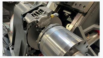
The mechanical disc brake on the C-Axis provides 140 ft-lb (190 Nm) of holding torque for off centre milling and drilling.
