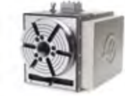
HRT210SP 4-AXIS COMPACT • 210 mm Platter • 100°/sec • Resolution 0.001°
