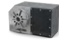
HRT160SS 4-AXIS HIGH SPEED • 160 mm Platter • 500°/sec • Resolution 0.001°
