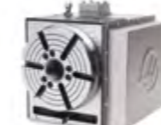
HRT310SP 4-AXIS COMPACT • 310 mm Platter • 75°/sec • Resolution 0.001°
