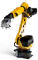
25kg CAPACITY ROBOT SYSTEM VF-1 to VF-5 UMC-400 to UMC-1000SS
