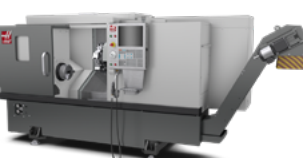
ST-15L BIG BORE LONG BED • Max Cut Ø 305 x L 826 mm • Bar Capacity 64 mm • A2-6 • 4,000 rpm • 20 hp • Chuck 210 mm
