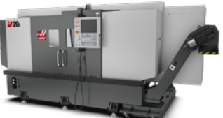
ST-20L LONG BED • Max Cut Ø 330 x L 1,080 mm • Bar Capacity 64 mm • A2-6 • 4,000 rpm • 20 hp • Chuck 210 mm
