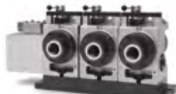
HA5C-3 4-AXIS • Torque 34 Nm • 0.001 to 200°/sec • Resolution 0.001°
